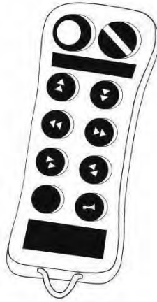
Figure 2.8 Remote control operator station
