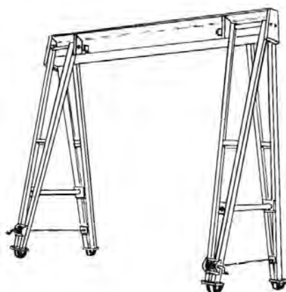
Figure 12.11 Self erecting gantry
