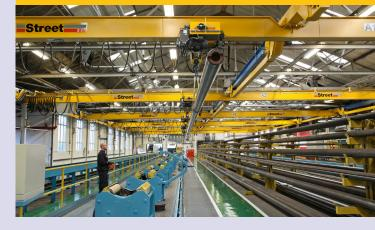
"Cranes are often an integral part of the manufacturing process, but with this project we have taken crane integration one stage further. These cranes have been engineered to enable both tooling and product to be handled safely, efficiently and flexibly, helping the company achieve greater responsiveness in their manufacturing operations."
